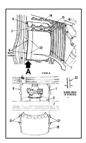
13. Check that seals (3, 10, and 20) at forward end of three segments (1, 9, and 19) fit against shroud (4) and do not overlap. Trim seals as needed.Gap between seals shall not exceed 0.06 inch.
