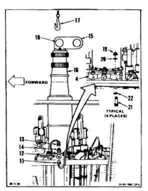
9. Tie rope guide line (23) around rotor shaft (16).
