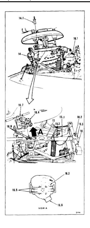
9.1. Torque aft bolt (16.1) as follows:
