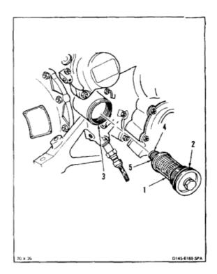
6. Lockwire filter (1) to transmission lug (6) lockwire (E231).
