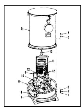
9. Remove all tape and barrier material from transmission (10).
