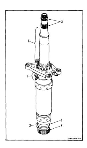
3. Blend out damage to enter section as shown.
