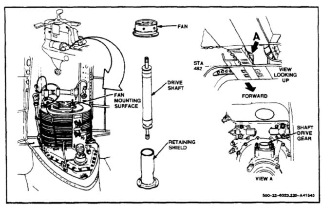
1. With retaining nut (1) of fan (2) facing up, set the fan on a firm surface.
