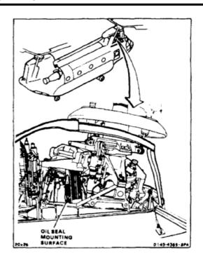
1. Clean seal retainer (1). Use dry cleaning solvent (E162) and cloths (E120). Wear gloves (E186).
