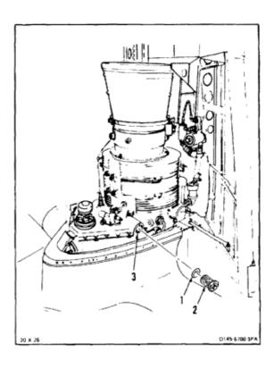
3. Lockwire screen (2) to transmission (4). Use lockwire (E231).
