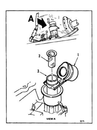
3. Check screen (2) for bits of metal and other debris. Retain debris for contamination analysis (Task 6-108).
