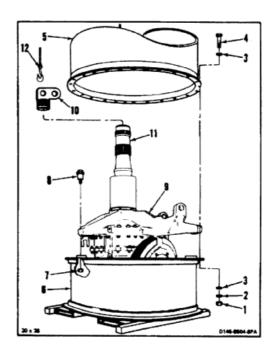
9. Remove all tape and barrier material from transmission (9).
