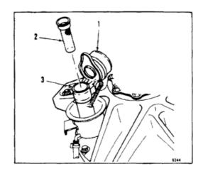
3. Check screen (2) for bits of metal and other debris. Retain debris for contamination analysis (Task 6-108).
