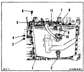
5. Remove 21 nuts (3) and washers (4) from around sump (1). Remove 14 bolts (6) and washers (12).
