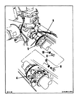
6. With aid of helper lift shaft (9) from between adapter assemblies (4 and 5). Remove shaft.
