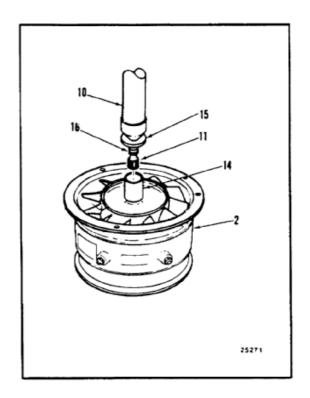
g. Half-fill splined cavity (17) in the fan drive gear with grease (E190.1). Insert the clean end of shaft (10) into the cavity. Gradually apply enough steady downward pressure to fully seat the shaft against snubber (18). Wipe off excess grease from around shaft and snubber (18). Check that balance flange (19) seats against the snubber.
