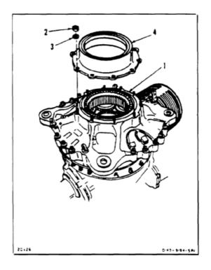
3. Check packing (5) around bottom of retainer (4) for cuts. It shall have no cuts.
