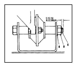
7. Rotate plates (4) to align hole (5) with lower of two mounting bolt holes in support (10).
