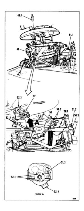
22.1. Loosen aft bolt (51.1) as follows:
