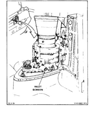
1. Remove lockwire from inlet screen (1).
