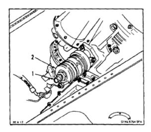
2. Remove lockwire from filter bowl (2). Remove bowl from housing (3).
