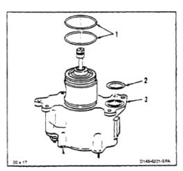
1. Install two packings (1) and packing (2) in pump (3).
