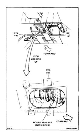
1. Install left or right mount (1), with bushing (2), in same way as forward drive shaft mount (Task 6-15).
