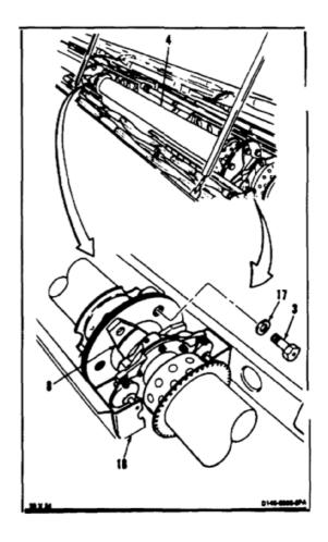
9. If shaft (4) is being replaced, install bolt (7), special washer (6) and nut (5) in adapter assembly (8). Remove bushing (10) from mount (19) on each side of adapter assembly.
