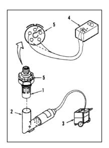
7. Remove test leads of multimeter (4) from chip detector (5).
