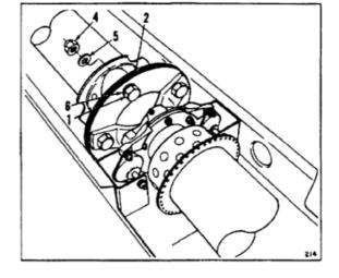
2. Rotate plates (2) to align hole (7) with lower of two mounting bolts (8).
