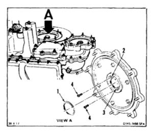
4. Cut a piece of lockwire (5) about **24 inches** long. Use lockwire (E232). Wrap ends of lockwire under heads of two screws (4).
