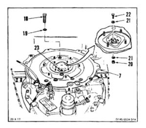
8. Lift cover (7) straight up from sump (24). Remove cover.
