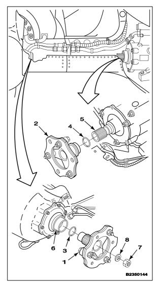
5. Install adapter assembly (1) in engine transmission output shaft (6). Wipe off excess grease with cloths (E120).
