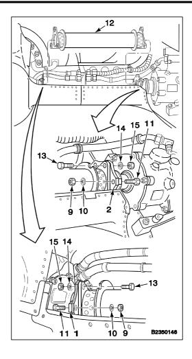
12. Have helper rotate blades to turn shaft (12) at least one full turn. Check that there is at least **0.125 inch** clearance between shaft and adapters (1 and 2) and the surrounding structure. Check for at least **0.5 inch** clearance to hoses and wires.
