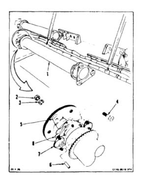
2. Turn bearing support housing (8) so that grease fitting (9) faces up.
