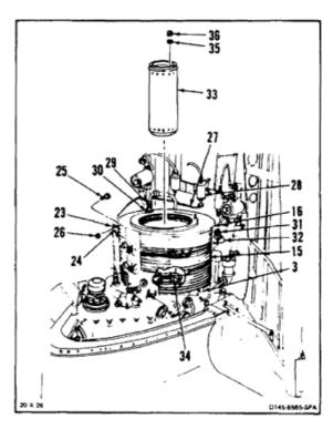
14. Lockwire three drain plugs (37) to oil cooler (4, 15, and 16). Use lockwire (E231).
