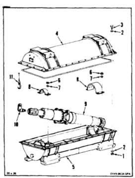
9. Remove all tape and barrier material from shaft (9).
