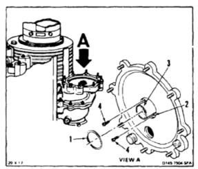
4. Cut a piece of lockwire (E232) (5) about **24** inches long. Wrap ends of lockwire under heads of two screws (4).
