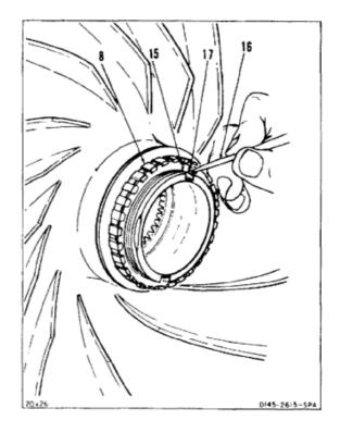
c. Install edge of screwdriver (16) in slot (17) and push retaining ring (15) clockwise. Ring shall expand under teeth of locknut (8) to lock.
