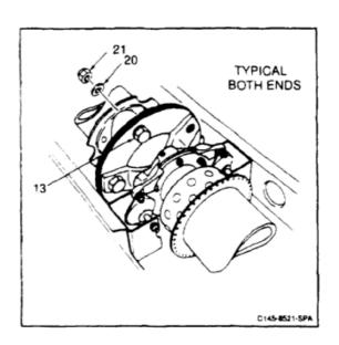
14. Coat two adapter assembly bolts (4) with oil (E254). Install bolts, special washers (3), and nuts (2).
