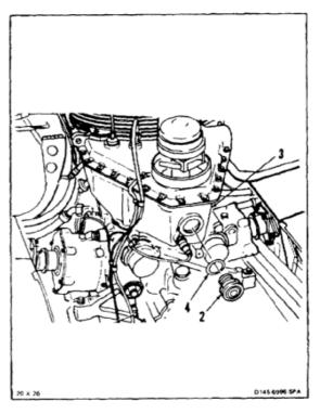
8. Lockwire sight gage (2) to temperature probe (5). Use lockwire (E231).
