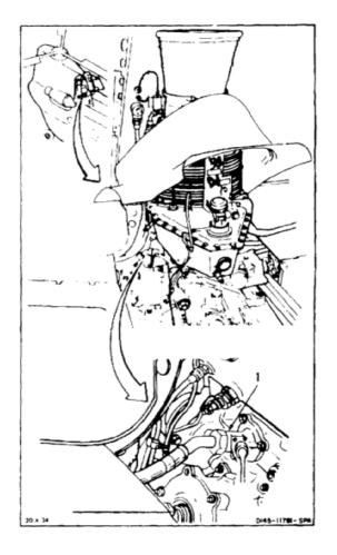
3. Remove and inspect chip detector plug (2) (Task 6-205). Install plug (Task 6-206).
