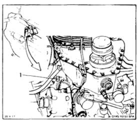
12. Remove and inspect chip detector plug (2) (Task 6-205). Install plug (Task 6-206).
