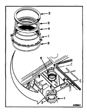
6. If retainer installation components were not finished in step 1, seal the installation as follows:
