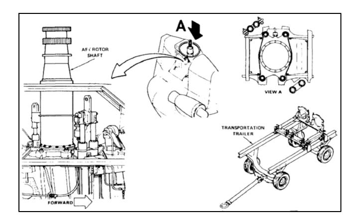
1. Cover slider shaft (1) with barrier material (E81) and tape (E388).
