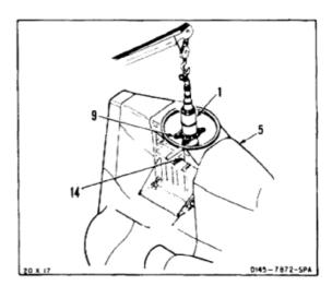
9. Turn bearing support (9) so that chip detector (15) and union (16) point forward. Align four mounting holes (17) in support (9) with holes (18) in structure (19).
