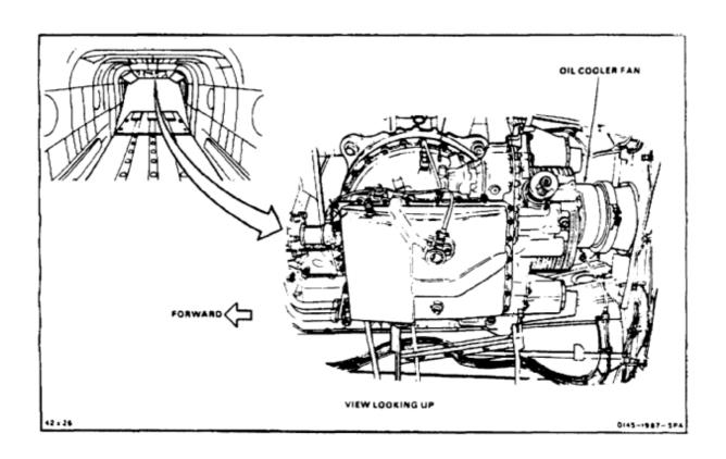
1. Loosen clamp (1) securing duct (2) to fan (3). Slide duct and clamp aft, off fan.
