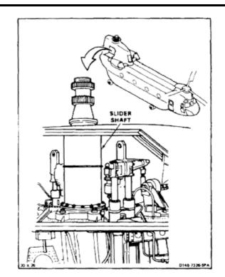
1. Remove 16 nuts (1) and washers (2) from base of slider shaft (3).
