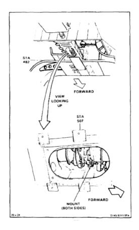
1. Remove either mount (1) in same way as forward drive shaft mount (Task 6-14).
