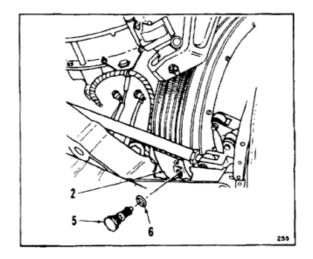
8. Lockwire valve (5) to nipple (7). Use lockwire (E231).
