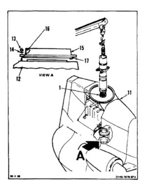
Be careful when handling seal. Seal is easy to damage.
