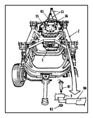
37. Cover splines (84) of rotor shaft (7) with barrier material (E80) and tape (E388).
