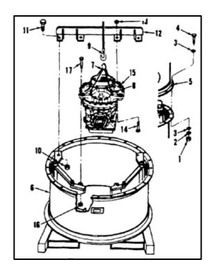
11. Remove all tape and barrier material from transmission (15).
