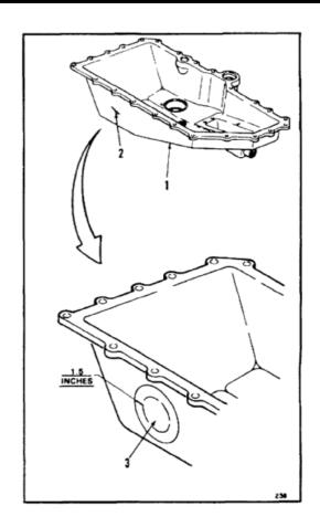
6. Cover sump (1) around cleaned area (4) with Teflon tape (E399) (5).
