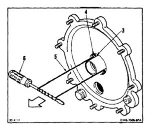
6. Remove packing (7) from transmission.
