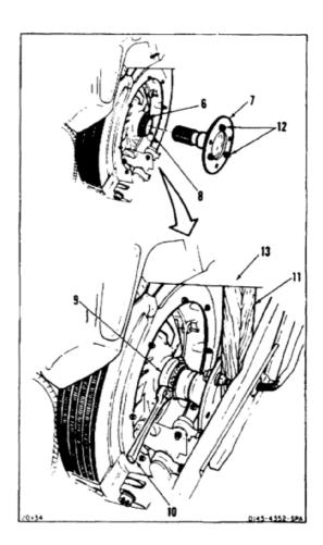
4. Remove adapter assembly (7). Remove locknut (6).
